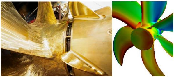
As a result of CFD (Computational Fluid Dynamics) analysis, this Short-Bodied & Specialized Design PBCF has demonstrated a fuel efficiency improvement of over 2.0% even on vessels already equipped with energy-saving fins and rudder bulbs. This significantly reduces CO2 emissions during vessel operations, contributing to our customers' environmental load reduction and operational cost savings.
